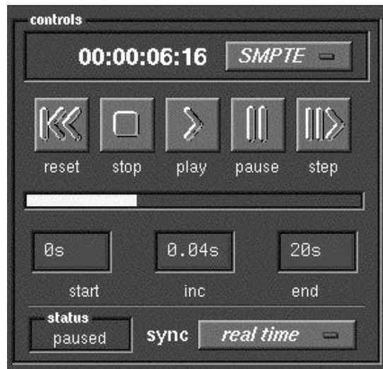
Figure 9-19: Conductor GUI, showing transport, timing and synchronisation controls. The user may set start, end and update (increment) times via text boxes. The time bar (centre) shows progress from start to end. Current time is displayed at the top (a variety of formats can be selected). Synchronisation can be selected from a number of available sources, and even changed while the system is running. A status box shows the current status, including synchronisation locking if the conductor is locked to an external sync source.
