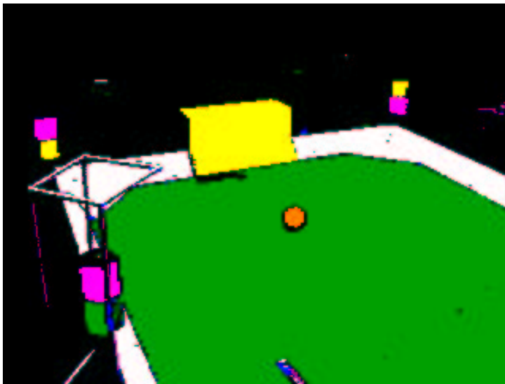
Figure 2.14: RGB output of the image in Figure 2.13 after segmentation by CMVision. (source: CMVision website)
