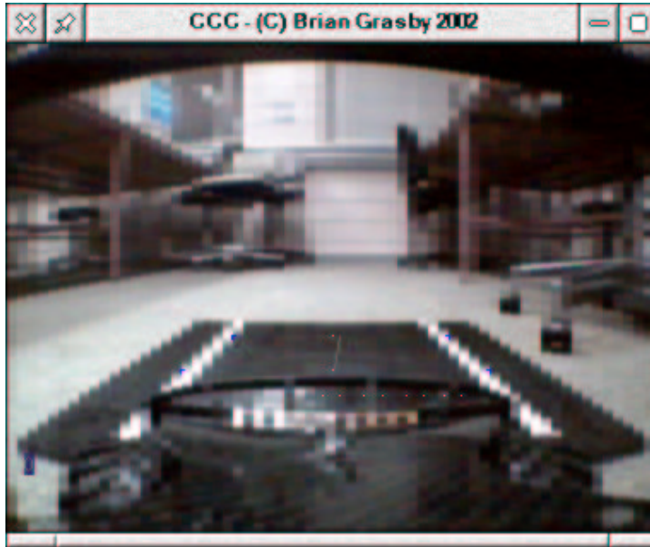
Figure 4.4: Results using an averaging filter with the block size set to 6 x 2 pixels. This block size was found to be the most efficient by Bruton (1999)
