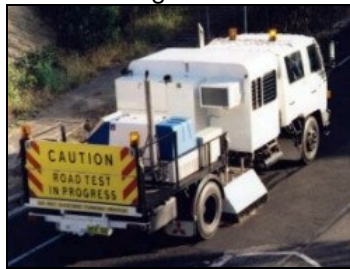
CSIRO Road Crack Vehicle.
