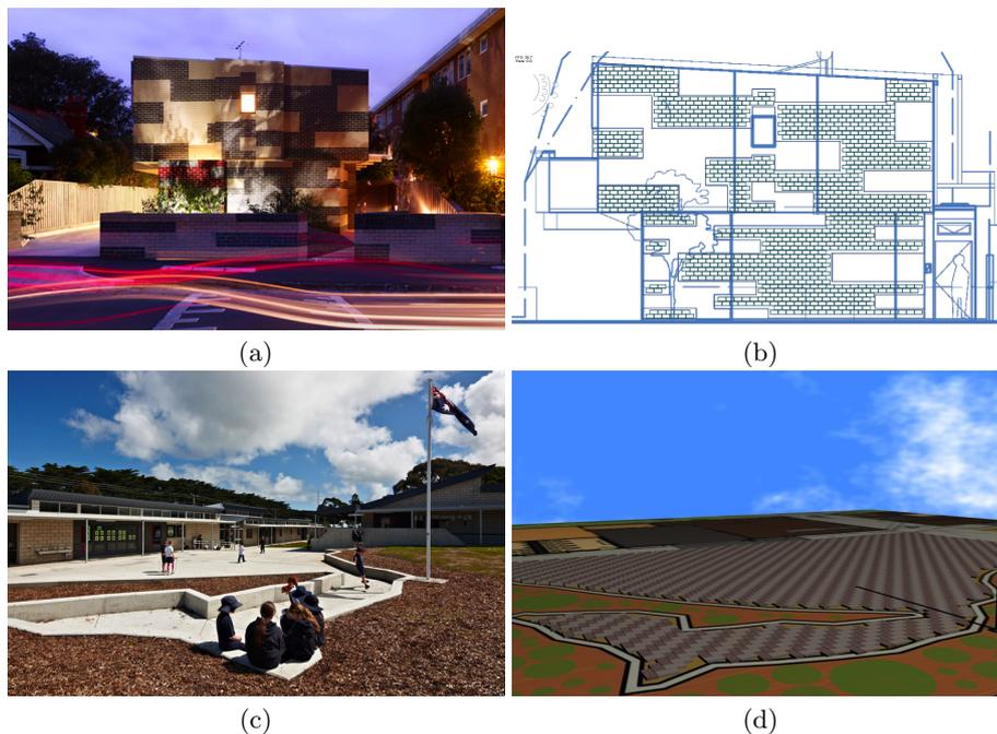
**Fig. 8.** Site photographs and tiling patterns overlaid on architectural plans. (a) Complex brickwork regions on East St. Kilda multi-housing development, Melbourne, Australia. Opat Architects 2011. (b) TILE screen grab of bricked regions. (c) Concreted region, Inverloch Primary School, Victoria, Australia. Opat Architects, 2011. (d) Sample 3D rendering of the irregular region paved with whole bricks.
