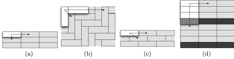
**Fig. 5.** Images of (a) stack-bond, (b) herringbone, (c) stretcher-bond bricks, (d) a stripe generated with a block of sub-tiles (cf. Figure 1c). These patterns are all generated using vector tiling. Vector axis alignments to generate these patterns from the base arrangements (illustrated in white) are shown.
