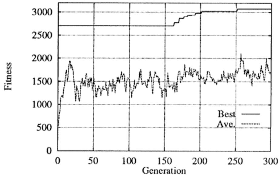
Figure 9: Evolution in binary adder
