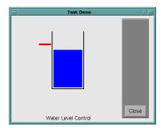
A controller for the water level in the tank needs to know the current water level and it needs to be able to set the valve. Our controller's input will be the water level error (desired water level minus actual water level) and its output will be the rate at which the valve is opening or closing. A first pass at writing a fuzzy controller for this system might be the following.
