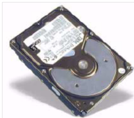
Hard Disk Drive (HDD) with magnetic moving head
