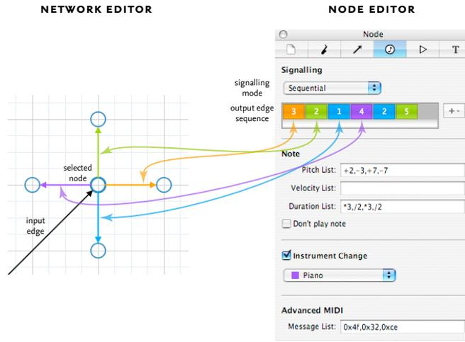
**Fig. 4.** Sequence editing. Output edges for the node selected in the network editor (left) are colour coded to match the numeric colour chips that specify the sequence of output edges in the node editor (right).
