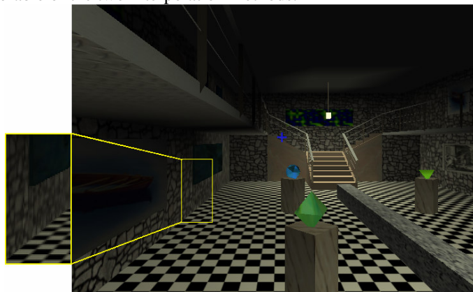
Figure 11: Frame rendered with linear interpolated region warping, tearing is no longer apparent.
