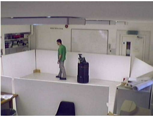
Figure 7: The robot environment in the wall-following experiment. The robot is programmed to track and follow a human demonstrator using its on-board camera; the input to the mirror system comes from the sonar sensors around its body.
