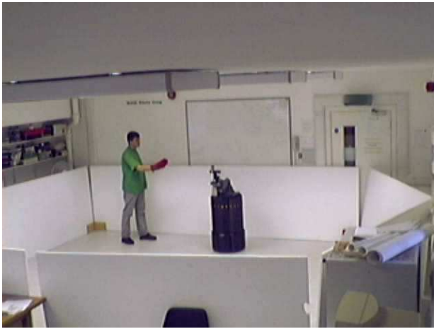
Figure 3: The robot Gillespie learns a wall-following task from a human demonstrator who actively demonstrates the task and explicitly influences the learning using hand signals.
