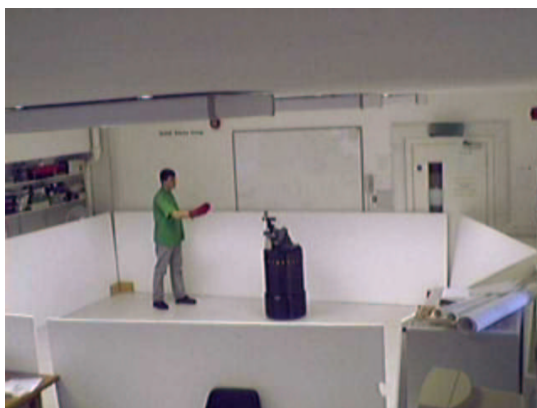
Figure 4.12: The physical wall-following experimental setup, where the demonstrator can explicitly signal to the robot.
