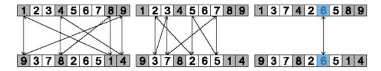
Step 2: copy alternate cycles into offspring
